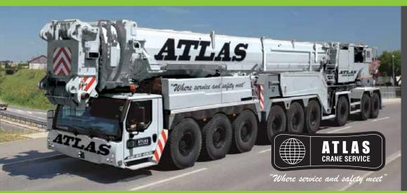
The key feature of the 9-axle LTM 1750-9.1 is that it can carry its entire telescopic boom on public roads. Its high load capacities and variable boom Systems enable it to cover a wide range of uses. In terms of its construction, this Liebherr mobile crane is designed for particularly short set-up times.
